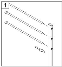
1. Insert the side bar into the tube and position at the desired location.
