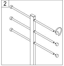
2. Secure the sift head onto the other end of the slide bar tightly in a clockwise direction.
