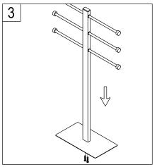
3. Install towel holder assembly onto the base and secure the bolt tightening with the allen wrench.
